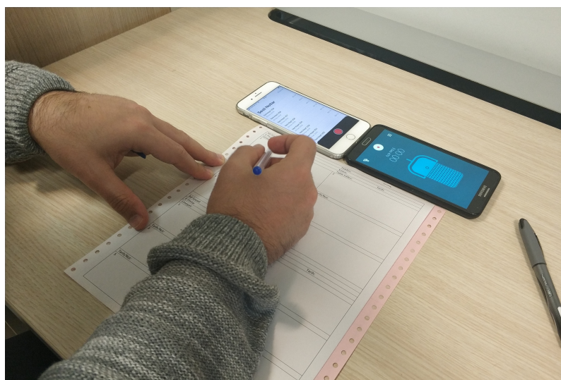
Figure 2.1 Two mobile phones are displayed in an experimental setup with a BIC Cristal ballpoint pen and thin paper with the auto-copy feature (To the right is a rollerball fine-point pen)
